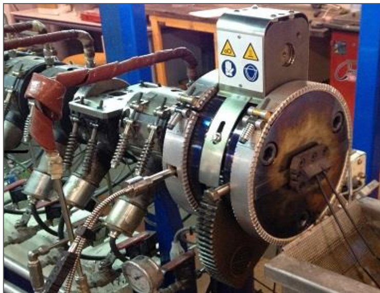
Elastomers and non melted plastics removed with filtration during extrusion phase
